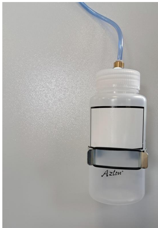
Figure 22: The condensate collection bottle for the air-conditioning unit
