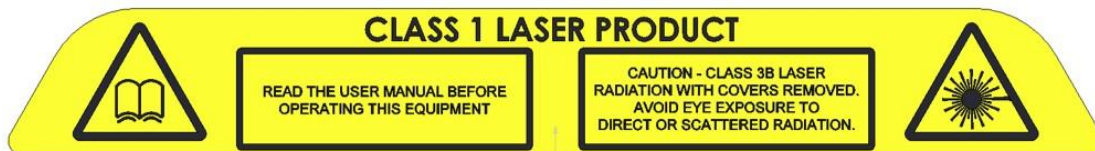
Figure 3: Laser safety label behind the front cover
