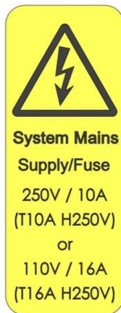
Figure 1: Electrical safety labels on the rear of the TeraCota core instrument
