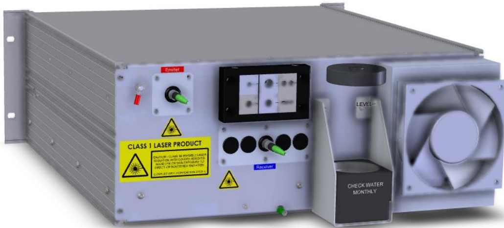
Figure 14: Rear view of the Optics Rack Assembly, showing cooling system reservoir and fan
