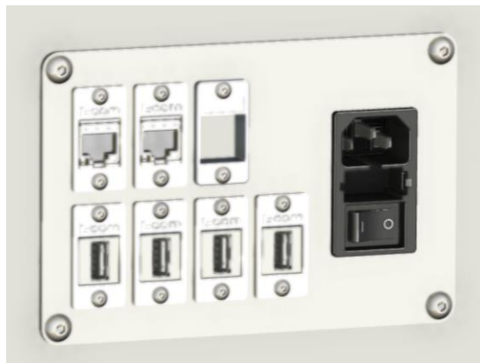
Figure 18: Bulkhead panel on the cabinet side
